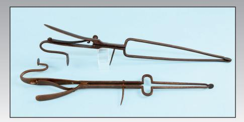
**363. RARE PAIR OF AMERICAN STEEL EMBER TONGS,** 18<sup>th</sup> century, complete with pipe tamper and functioning sprung hinge. Tongs like this were used to take glowing embers to light a smoker's pipe. Length 18 <sup>5</sup>/<sub>8</sub> in. 900/1,200
